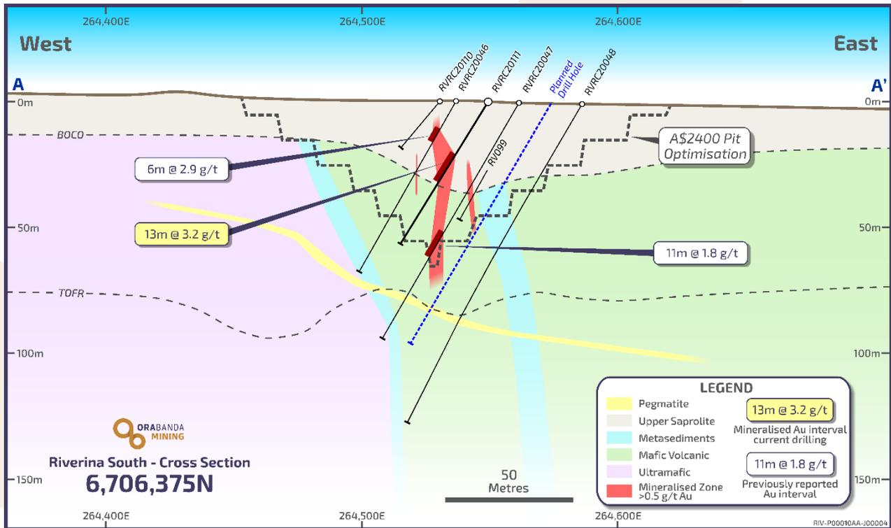
Figure 4 – Cross Section A\_A of recent drilling
