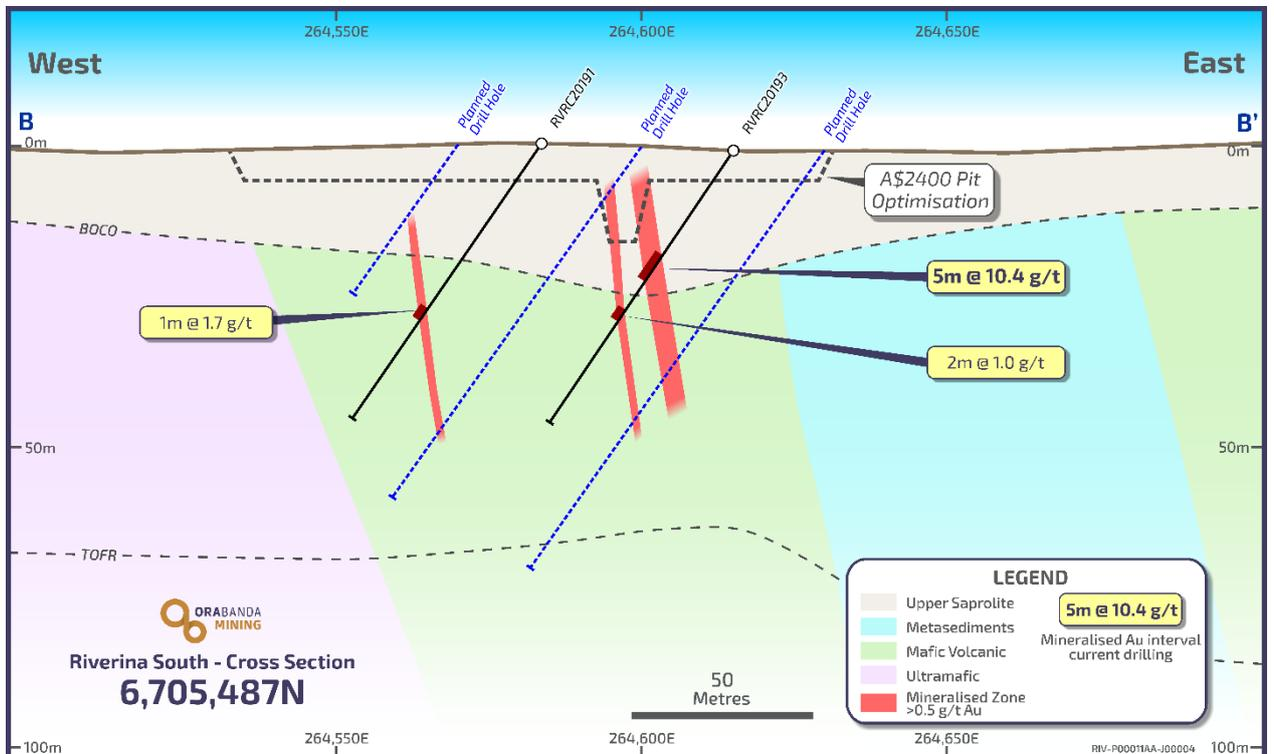
Figure 5 – Cross Section B\_B of recent drilling – the most southern RC drill section
