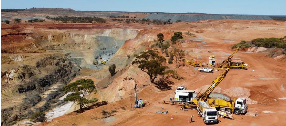
Figure 8 - Looking south over Sand King toward Missouri, with 2 diamond drill rigs deployed on the Sand King underground program
