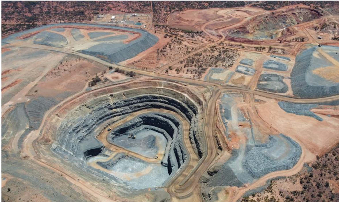
Figure 1 - Looking north over Missouri Open Pit to Sand King Open Pit and highlighting the reduced strip ratio in the Missouri Open Pit
