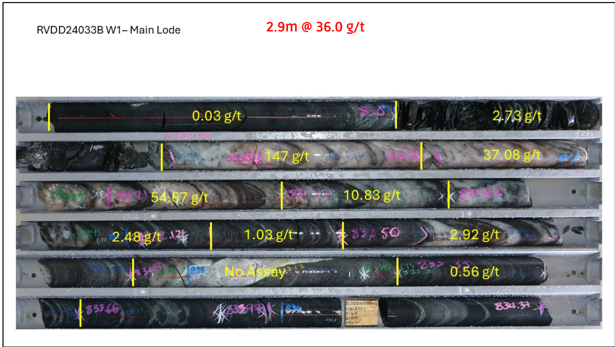
Figure 3 – Core photos of RVDD24033B – W1 – showing assay data on a consistent high-grade quartz lode intersected in good ground condition and at its anticipated position. This is a wedge hole that achieved 60 vertical metres separation from the parent hole shown below.
