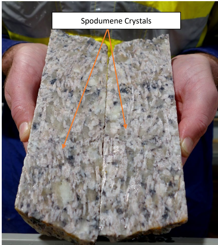
Figure 7 - Hole 1 (FLLIDD2301) section of basal LCT pegmatite showing abundant spodumene crystals
